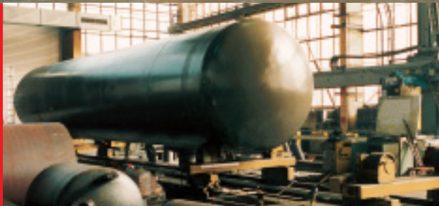
New epoxy coated tank.
