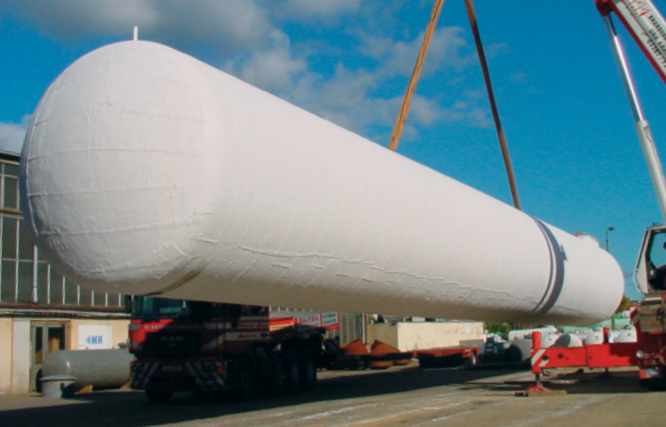
Overhauled custom tank with bitumen coating.
